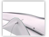
6. Thread cable support through eyelet.
