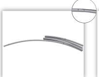
1. Start connecting the different sections of the frame by pushing the ends together.
